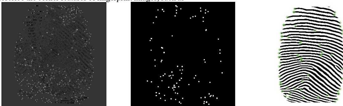
Fig.1 Fingerprint feature point detection and extraction example
